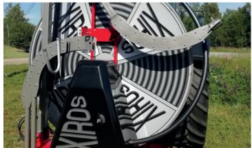
The Xiros drain cleaner feeds the rinsing hose into the drain pipe and rinses it with a pressurized water jet. The rinsing hose is 500 meter long, and the three-dimensionally moving drainage guide arm leads the rinsing hose to the drain. The large maneuverability of the drainage guide arm facilitates the positioning and rinsing work.
